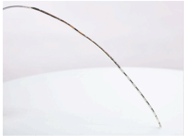
Fig. 1. The Freedom-8A SCS neurostimulator with 8 electrodes, a microchip, and a miniature receiver embedded into the inner lumen of the stimulator body.
