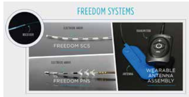
Fig. 1. Freedom SCS/PNS systems. SCS, spinal cord stimulation; PNS, peripheral nerve stimulation.
