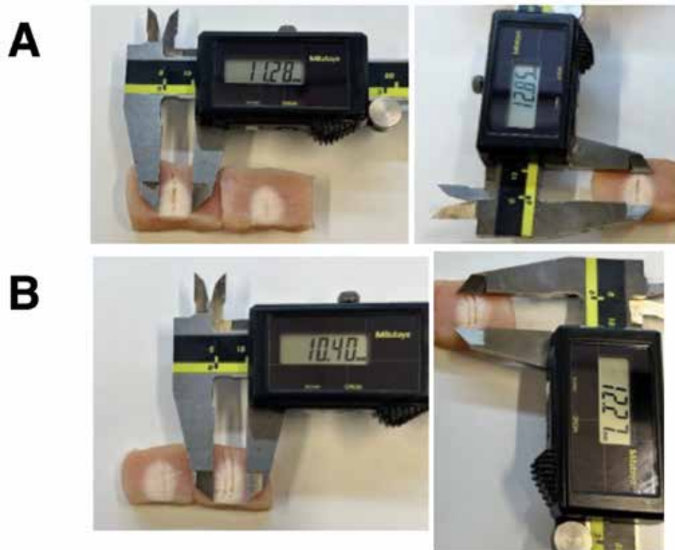
Fig. 6. Experimental bench-top comparison demonstrating an approximate 23% larger ellipsoidal volume in tissue samples for the Nimbus electrode in monopolar mode (A) vs standard 18G electrodes in bipolar mode (B). Both procedures were conducted at 85°C for 90 seconds.
